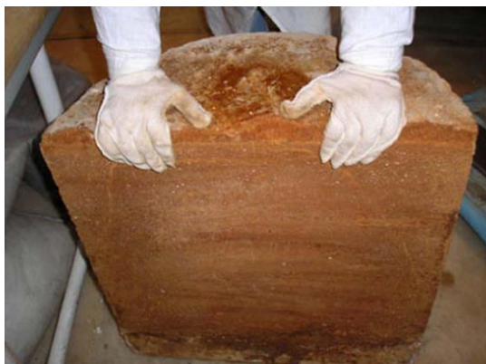
Fig. 1. MPP matrix obtained by solidification of M-2 (PA Mayak, Russia).
